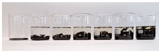
NeoTerra Aquafix™ pellets in the beginning of the water holding capacity (WHC) test. Photographs taken each hour during first 0–6 hours.
